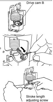
(3) Turn the cam of this side by hand to adjust the dial (%).
