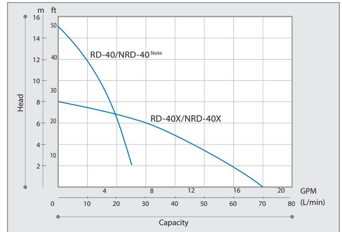
Note: Do not exceed 6.6 GPM in operation, or cavitation may take place. The above curves are based on operation with a 5V external control signal.
