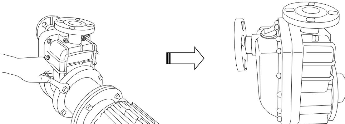
3. Remove the three hex socket cap head bolts that secure the rear casing support to the rear casing.
