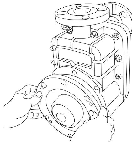
6. Remove the remaining nuts securing the front and rear cases and separate.
