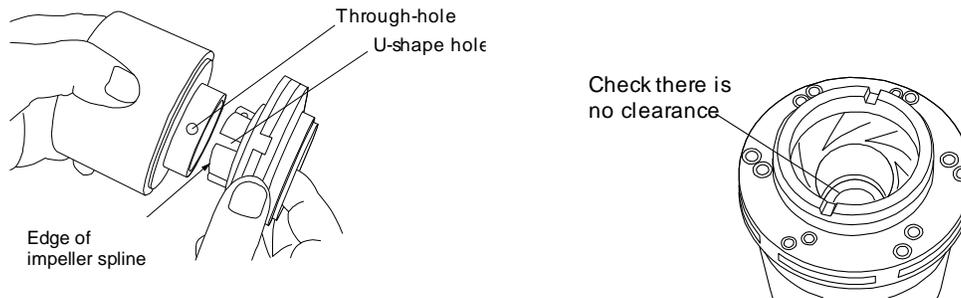
8. Place O-ring into front casing then slide the impeller magnet assembly onto the spindle. Take care not to chip bearing or spindle edges when re-assembling.
