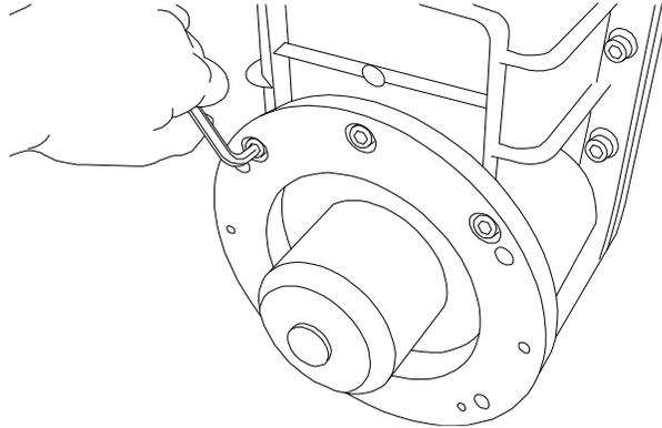
4. Remove all cover caps and the five nuts securing the front casing. At this point any remaining liquid can be drained from the pump.
