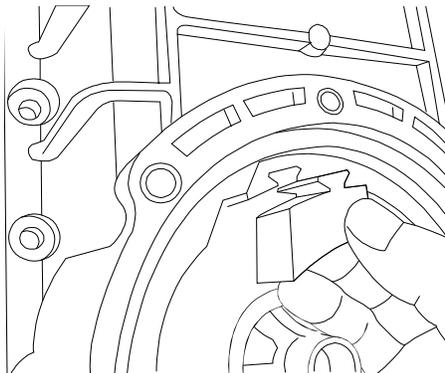
5. Lay the rear case on flat surface, impeller side down. Place front case and plate assembly on rear case. Temporarily tighten the hex socket head bolts to secure the assembly and prevent the o-ring and gasket from moving.
