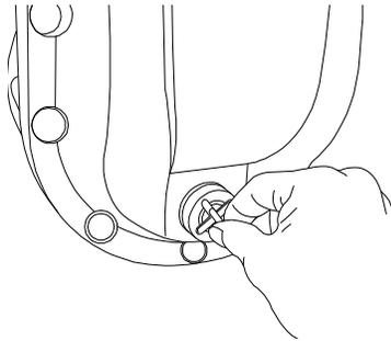
2. Next, loosen the four hex head bolts on the motor bracket to remove the pump head from the motor.
