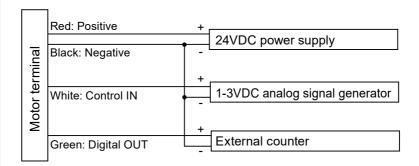
5 Use an external fuse (e.g 3A) to protect the motor
