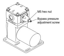
2 Close the ball/needle valve slowly to give the back pressure to the pump where the bypass valve starts opening
