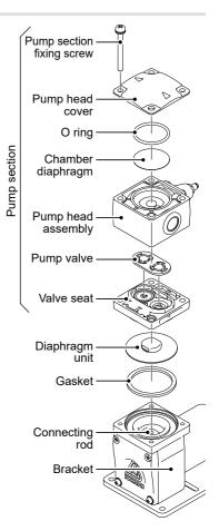
5 Push down the Diaphragm unit until it bottoms out
